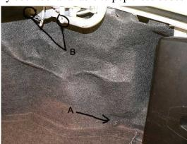
screwdriver. You will also need to remove the cargo net hook "A". It just unscrews.
